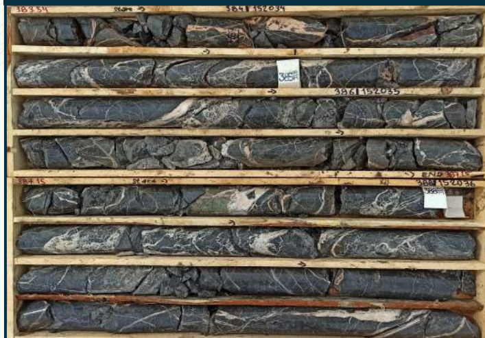
AAD-102: (60 to 67m) Magmatic hydrothermal breccia of quartz monzonite/dacite porphyry; strong silica and magnetite alteration with moderate phyllic. Locally elevated in both Au, Cu.
