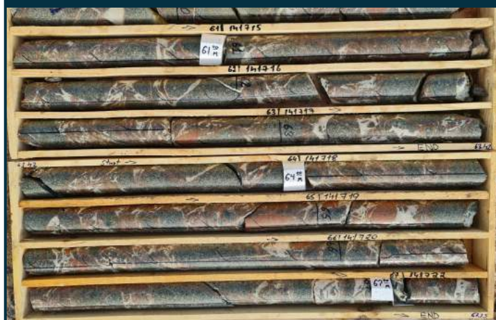
AAD-102: (60 to 67m) Magmatic hydrothermal breccia of quartz monzonite/dacite porphyry; strong silica and magnetite alteration with moderate phyllic. Locally elevated in both Au, Cu.
