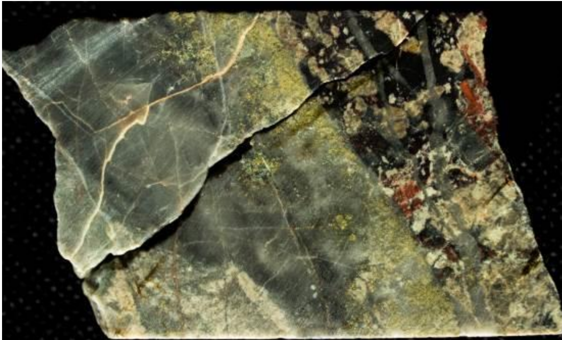
Figure 26 - Drill Core Photo showing visible gold in BKD-231; 2,200 g/t Au over 1 m
