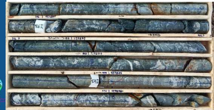
Mineralized epithermal and hydrothermal breccia (black/red) surrounded by phyllic alteration utilizing the contact between volcanic breccia and andesite
