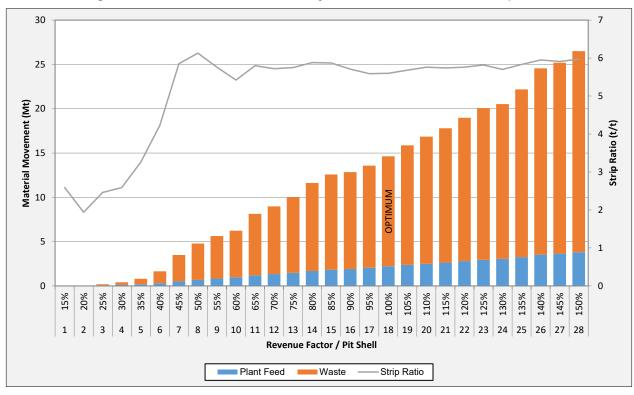
Figure 16-9 Altan Nar Price Sensitivity – Plant Feed, Waste and Strip Ratio
