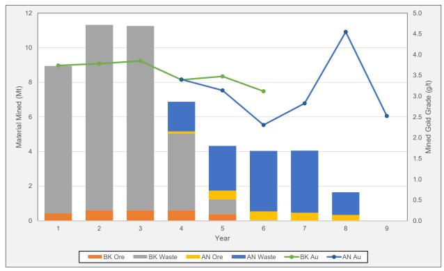
Figure 16-33 Production Schedule: Plant Feed and Waste Rock
