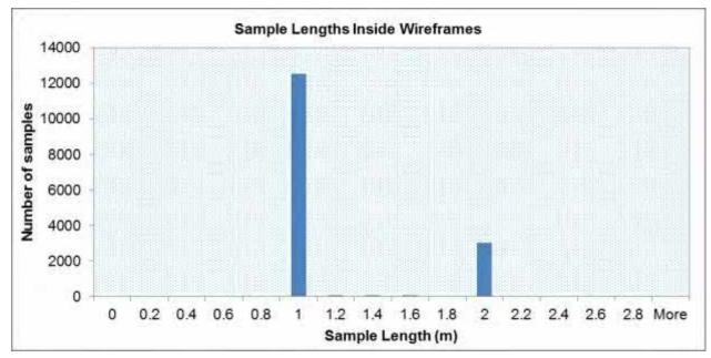
Surpac software was then used to extract 'best fit' one meter down-hole composites within the intervals coded as 'domain' intersections. This method adjusts the composite length within intersections to eliminate "rejected" samples that can occur when fixed length compositing is used. A minimum length of 50% was used due to the numerous very narrow intersections. This allowed a composite to be generated for intersections as narrow as 0.5 m.
