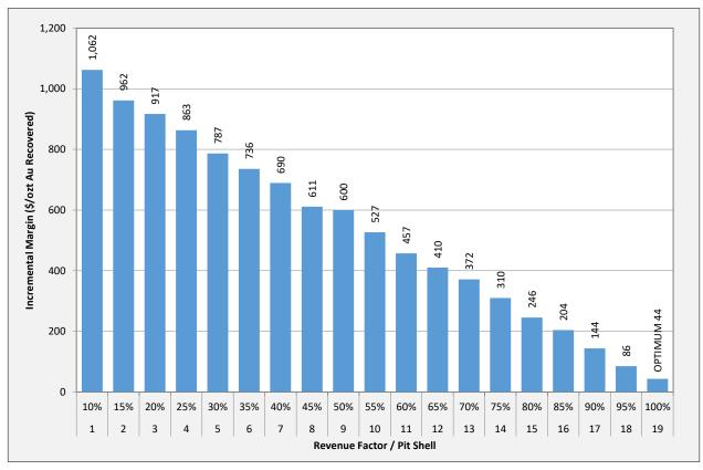
Figure 16-14 Bayan Khundii Shell Analysis - Incremental Margin
