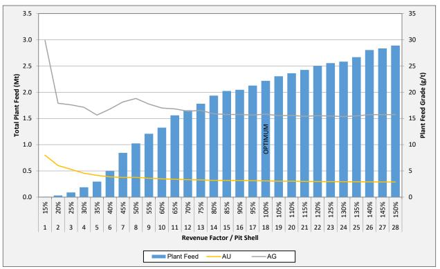
Figure 16-16 Altan Nar Shell Analysis - Plant Feed & Grade
