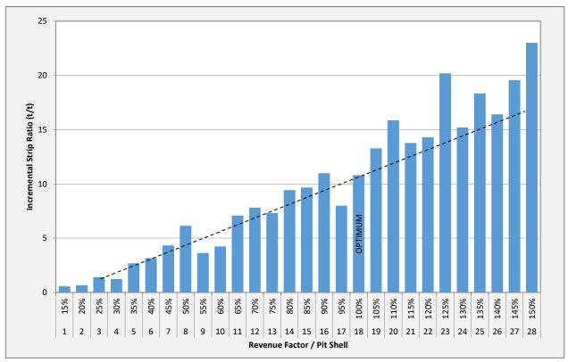
Figure 16-17 Altan Nar Shell Analysis - Incremental Strip Ratio
